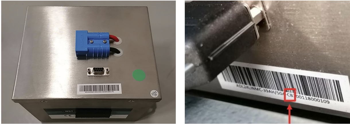
Figure 1.4. You can tell if the battery has CAN bus communication connection by the extra (black) connector and the letters “CB” in the serial number.
